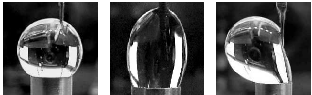
FIG. 7: Left: ideal spherical drop (3.5 ml), Center: attracted oblong drop (7 ml), Right: repulsed drop (5 ml).
